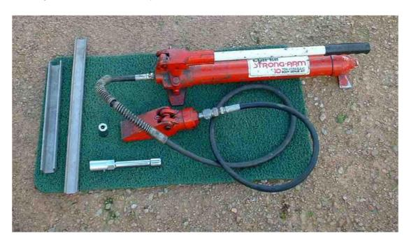
The front stiffener (spark plug socket and short half inch socket extension) was resting between the forward chassis cross member and lower block, to stop forward movement on engine mounts.
