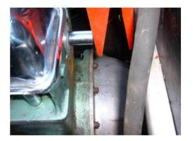
Even with the full half ton pressure to depress the plug inwards it needed the lower forward jaw to be hit with a heavy masons hammer to cause the core plug to indent and open, (short, sharp, and hard) this was done 4 times moving the socket in a circle around the center of the plug, the plug "dome " this way was flattened (reduced) 2mm.
